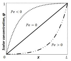
Fig. 1. Boundary conditions and solution profiles as a function of the Peclet number.
