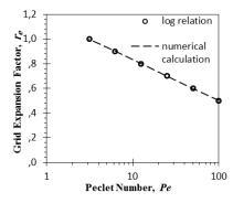
Fig. 4. Grid expansion factor  $r_e$  as a function of logarithm of the Peclet number Pe
