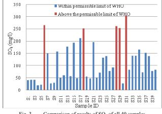
Fig. 3. Comparison of results of SO<sub>4</sub> of all 40 samples
