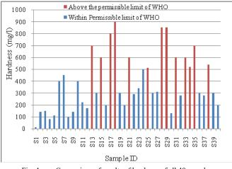
Fig. 4. Comparison of results of hardness of all 40 samples
