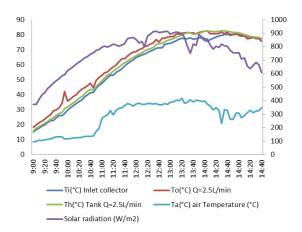
Fig. 8. Hot Solar intensity and various temperatures of solar collector at flow rate 2.5L/min.
