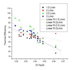
Fig. 7. Solar collector efficiency curve at four flow rates for water.
