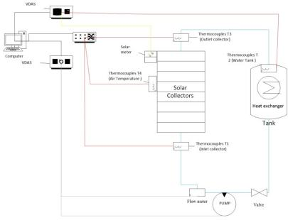
Fig. 1. Schematic of the experimental set-up.
