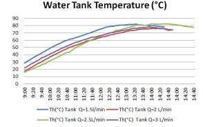
Fig. 6. Hot stored water at different flow rates.
