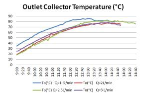
Fig. 5. Outlet Temperature at different flow rates.
