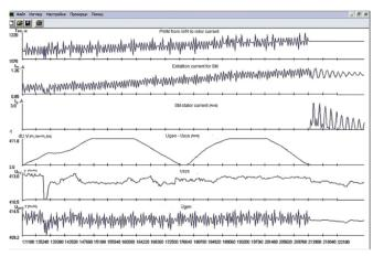
Fig. 14. Entering parallel of SG with power system – two cicles of dU[RMS] by excitation system sliding control.
