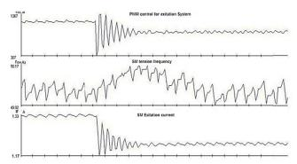
Fig. 13. Impact of the excitation current on the idle generator frequency
