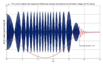
Fig. 8. Full cycle of relative rotor speed and differences between the system and generator voltage with 5% sliding
