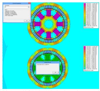
Fig. 4. Model of SG 400kVA / 6,3kV (lower image: resistance torque)
