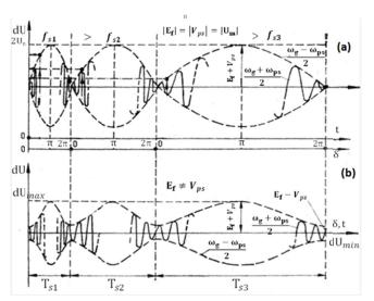
Fig. 3. The synchronization process – diagrame of the informative parameter dU for (a)  $|E_f| = |V_{ps}|$  and  $\omega_s \neq 0$ , (b) for  $|E_f| \neq |V_{ps}|$  and  $\omega_s \neq 0$  for three different sliding frequencies.
