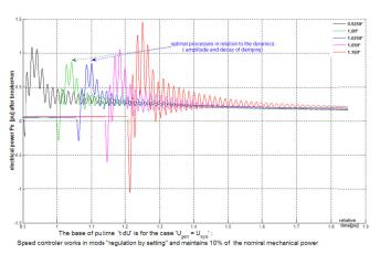
Fig. 12. The electrical power  $P_e[pu]$  in the synchronization process with excitation control for the limit and nominal values of  $I_{rnl}$
