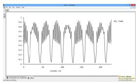
Fig. 5. The induction distribution in the air gap of the machine
