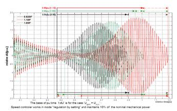
Fig. 10. Dependence of sliding period  $T_{s}[pu]$  by nominal and limits values of excitation current  $I_{fnl}$
