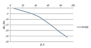
Fig. 6. Changes in the torque resistance of the turbine shaft as a function of the generator output current
