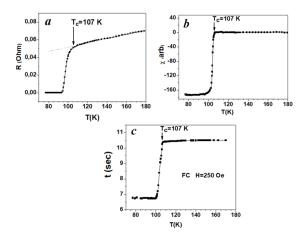
Fig. 2. The temperature dependence of electric resistance R (a), magnetic susceptibility  $\chi$  (b) and oscillation period t (c) of superconducting sample  $\mathrm{Bi}_{1.7}\mathrm{Pb}_{0.3}\mathrm{Sr}_2\mathrm{Ca}_2\mathrm{Cu}_3\mathrm{O}_{10-\delta}$  (2223) suspended on a thin elastic thread and making axial-torsional oscillation in transverse magnetic field.
