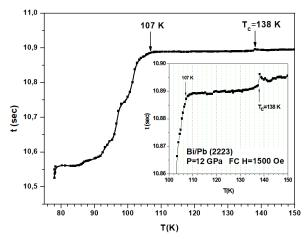
Fig. 8. Dependence of *t*-period on temperature T of superconducting sample suspended on a thin elastic thread and making axial-torsional oscillation in transverse magnetic field, at P~12GPa.
