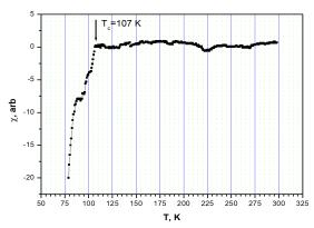
Fig. 1. Dependence of magnetic susceptibility  $\chi$  on temperature for Bi-Pb-Sr-Ca-Cu-O sample.
