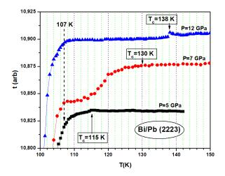
Fig. 10. Dependence of period t on temperature T of superconducting sample suspended on a thin elastic thread and making axial-torsional oscillation in transverse magnetic field, at  $P{\sim}5$ GPa,  $P{\sim}7$ GPa and  $P{\sim}12$ GPa.
