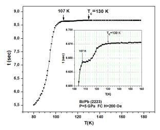
Fig. 6. Dependence of period t on temperature T of superconducting sample suspended on a thin elastic thread and making axial-torsional oscillation in transverse magnetic field, at P~7GPa.
