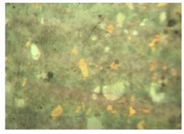
Fig. 7. Sample is compacted at pressure P=7GPa. The figure is taken at x350 magnification.
