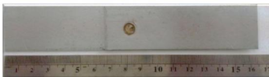
Fig. 3. Resistance spot welded specimen
