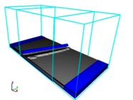
Fig. 6. Numerical simulation sample result, scouring hole beneath inclined pipe,  $\theta$ =130°
