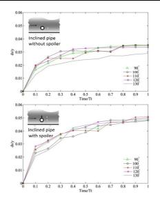
Fig. 10. Scouring progress beneath the inclined pipes, e/D=0.2
