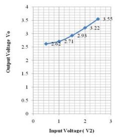
Fig. 3. Test results for Vt = 4V, V1 = 2.5V
