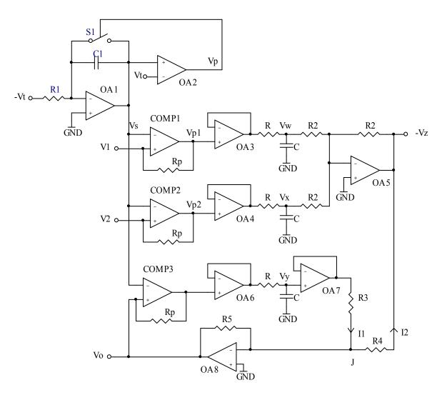
Fig. 1. Circuit diagram for the square root of the sum of two squared voltages
