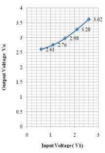
Fig. 4. Test results for Vt = 4V, V2 = 2.5V
