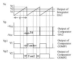
Fig. 2. Associated Waveforms of Figure 1
