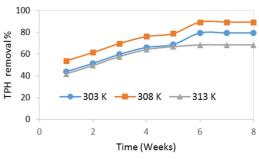
Fig. 5. Effect of operating temperature on TPH removal.
