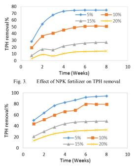
Fig. 4. Effect of activated sludge, NPK fertilizer and coconut shell powder on TPH removal
