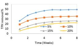
Fig. 1. Effect of coconut shell powder addition on TPH removal
