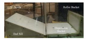
Fig. 1. Modified stilling basin with depression bucket
