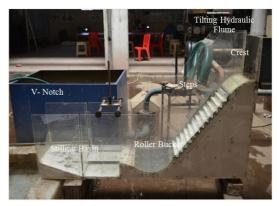
Fig. 2. Hydraulic model of the ogee rofile stepped spillway
