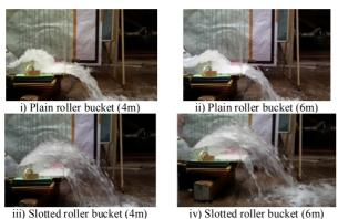
Fig. 3. Hydraulic jump on roller buckets without stilling basin
