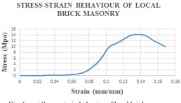
Fig. 1. Stress-strain behavior of local brick masonry
