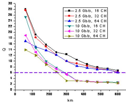
Fig. 5. Changing the Q factor for length of the amplifying section 60 km.
