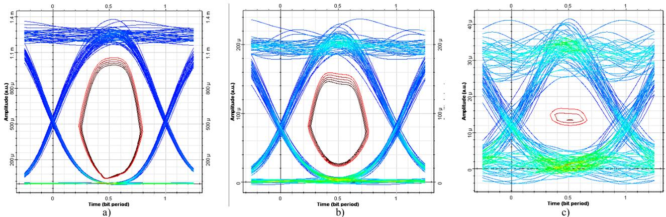
Fig. 8. The eye diagram for flow rate per channel 2.5 Gb/s and 16 DWDM channels: a) 80 km, b) 240 km, c) 400 km.
