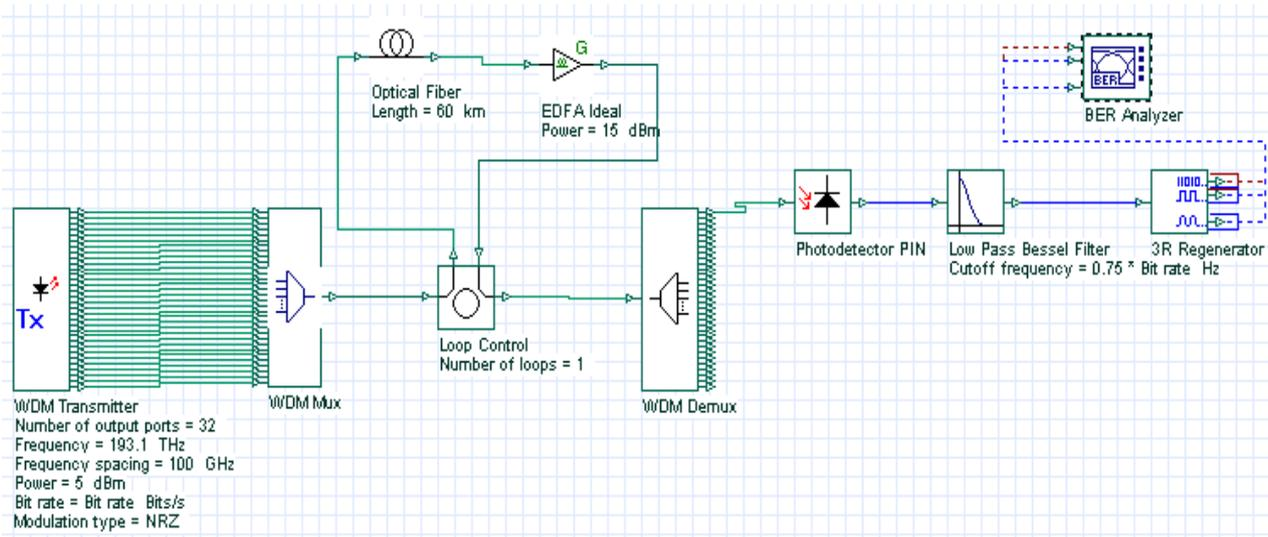
Fig. 2. 16-channels DWDM network.
