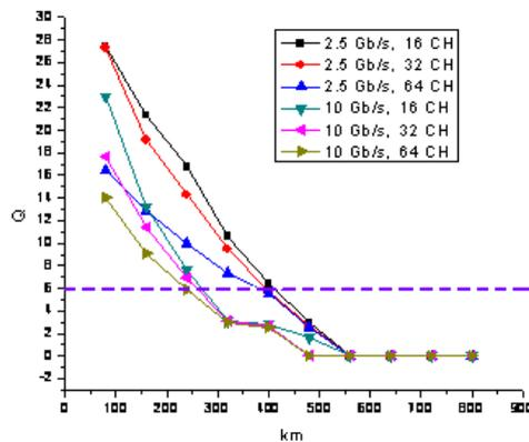
Fig. 7. Changing the Q factor for the length of the amplifying section 80 km.
