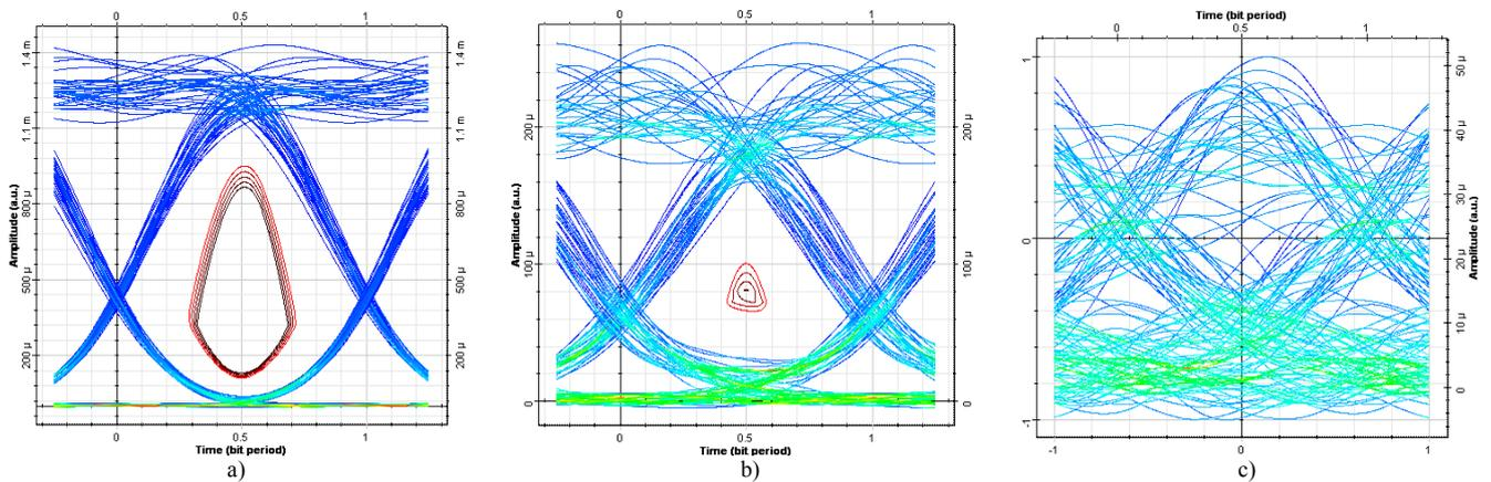
Fig. 12. The eye diagram for flow rate per channel 10 Gb/s and 32 DWDM channels: a) 80 km, b) 240 km, c) 400 km.
