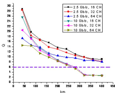
Fig. 3. Changing the Q factor for length of the amplifying section 40 km.
