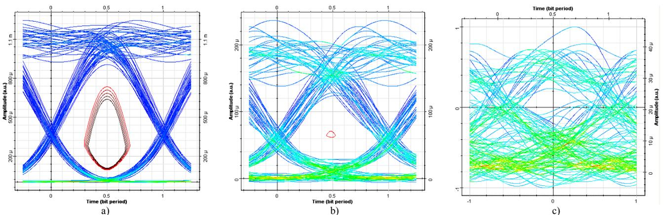
Fig. 13. The eye diagram for flow rate per channel 10 Gb/s and 64 DWDM channels: a) 80 km, b) 240 km, c) 400 km.
