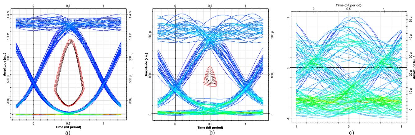
Fig. 11. The eye diagram for flow rate per channel 10 Gb/s and 16 DWDM channels: a) 80 km, b) 240 km, c) 400 km.
