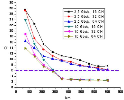
Fig. 6. Changing the Q factor for length of the amplifying section 70 km.
