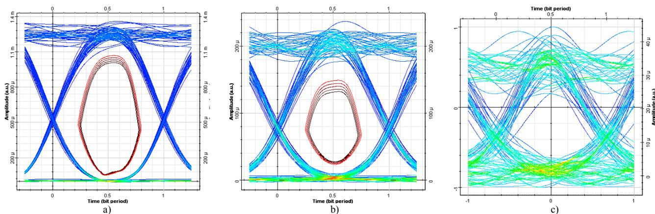
Fig. 9. The eye diagram for flow rate per channel 2.5 Gb/s and 32 DWDM channels: a) 80 km, b) 240 km, c) 400 km.
