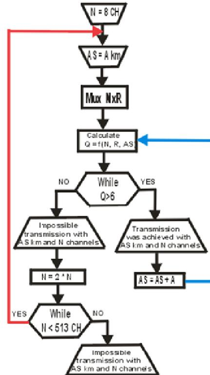
Fig. 1. Algorithm for the evaluation of quality of DWDM transmission network during the design stage.
