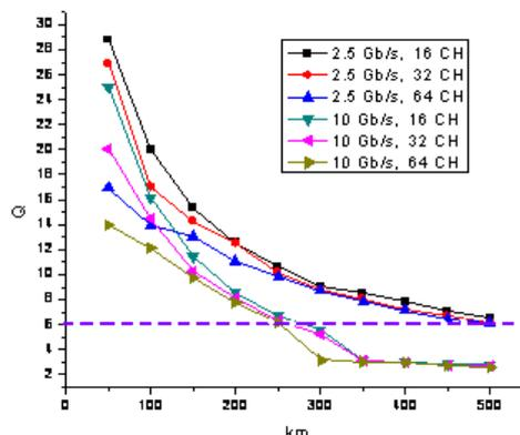
Fig. 4. Changing the Q factor for length of the amplifying section 50 km.
