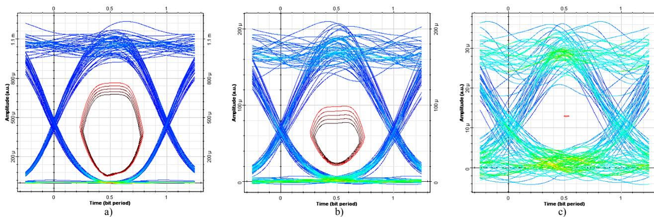
Fig. 10. The eye diagram for flow rate per channel 2.5 Gb/s and 64 DWDM channels: a) 80 km, b) 240 km, c) 400 km.
