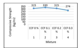
Fig. 4. Coir fiber paving block compressive strength graph at the age of 14 days
