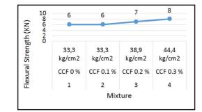
Fig. 6. Coir fiber paving block flexural strength graph at the age of 14 days
