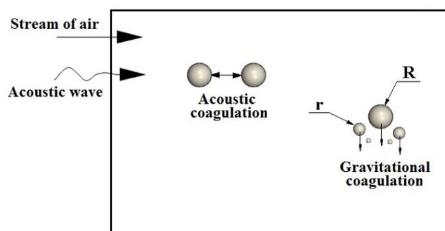
Fig. 1. Aerosol particles coagulation process
