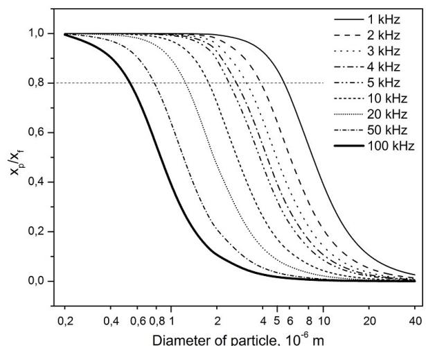
Fig. 2. Amplitude ratio as a function of the frequency of the acoustic field and the diameter of particles
