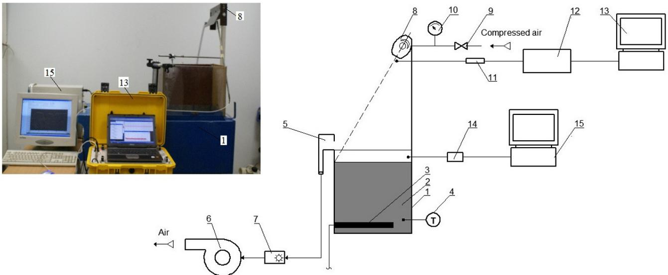
Fig. 3. Experimental stand: 1 – bath, 2 – liquid, 3 – heater, 4 – thermometer, 5 – side exhauster, 6 – fan, 7 – variable-frequency drive, 8 – blower and acoustic wave generator, 9 – valve, 10 – pressure gauge, 11 – hydrophone, 12 – data storage, 13, 15 – computer, 14 – temperature and humidity meter
