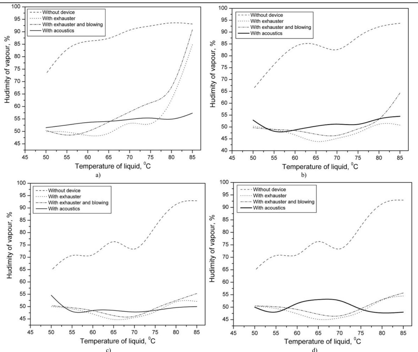
Fig. 6. Humidity of air measured at different distances from liquid surface as function of the liquid temperature and air removal method: a) – 0 mm distance (edge of the bath); b) – 100 mm distance above the bath; c) – 200 mm distance above the bath; d) – 300 mm distance above the bath
