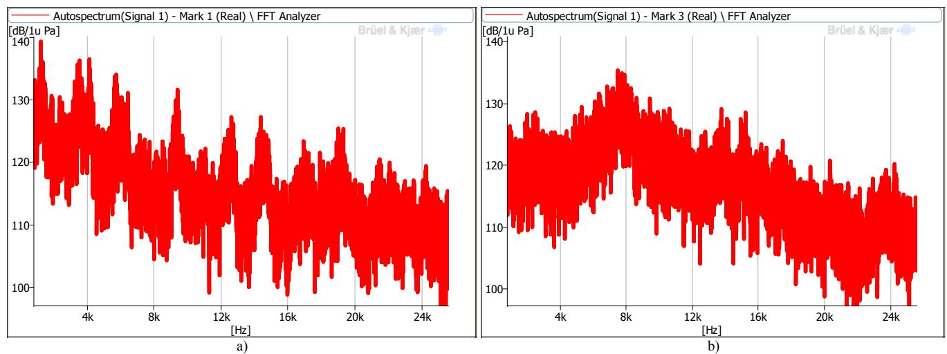
Fig. 5. Sound pressure level spectrum of acoustic wave generator when nozzle and resonator diameters ratio was equal to: a) – 1:2, b) – 1:5
