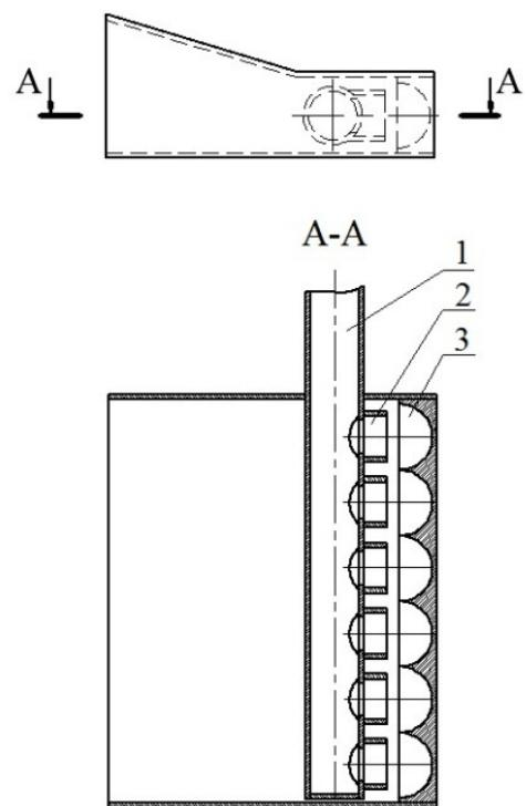
Fig. 4. Scheme of the acoustic wave generator: 1 – collector, 2 – nozzle, 3 – resonator
