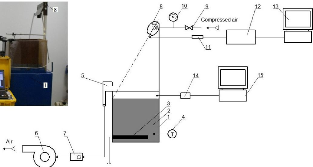
Fig. 3. Experimental stand: 1 – bath, 2 – liquid, 3 – heater, 4 – thermometer, 5 – side exhauster, 6 – fan, 7 – variable-frequency drive, 8 – blower and acoustic wave generator, 9 – valve, 10 – pressure gauge, 11 – hydrophone, 12 – data storage, 13, 15 – computer, 14 – temperature and humidity meter
