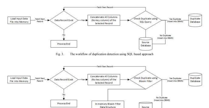
Fig. 4. The workflow of duplication detection using bloom filter-based approach
