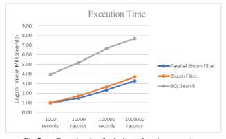
Fig. 7. Execution time for duplicate detection comparison
