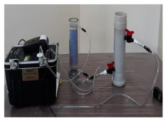
Fig. 1. Method of radon concentration measurement.
