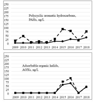
Fig. 5. Evolution per year of: PAHs (up); AOXs ( $\mu$ g/L) (down). Raw wastewater (squares-striped line); treated wastewater (dots-continuous line).
