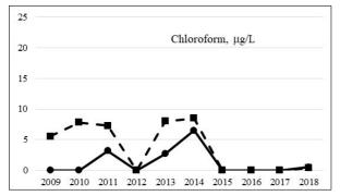
Fig. 7. Evolution per year of chloroform. Raw wastewater (squares-striped line); treated wastewater (dots-continuous line).
