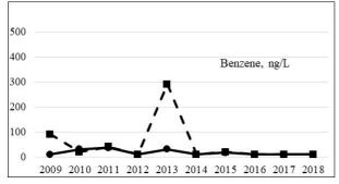
Fig. 6. Evolution per year of benzene. Raw wastewater (squares-striped line); treated wastewater (dots-continuous line).
