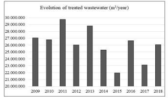
Fig. 2. Evolution per year of flow of wastewater in La Golondrina WWTP during 2009-2018.
