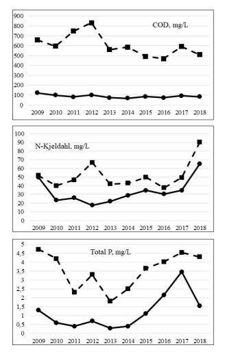
Fig. 3. Evolution per year of: COD (up); Kjeldahl N (middle); Total P (down). Raw wastewater (squares-striped line); treated wastewater (dots-continuous line).
