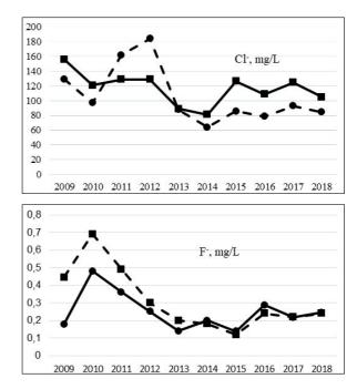
Fig. 4. Evolution per year of: Cl<sup>-</sup> (up); F<sup>-</sup> (down). Raw wastewater (squares-striped line); treated wastewater (dots-continuous line).
