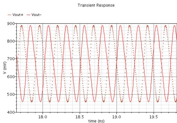
Fig. 6. The output voltage of the proposed oscillator
