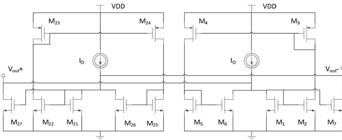
Fig. 5. Current mode LC oscillator based on the active inductor
