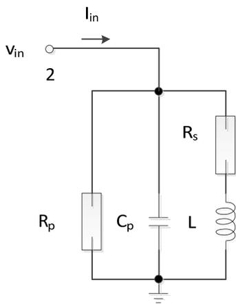
Fig. 3. The admittance looking into port 2
