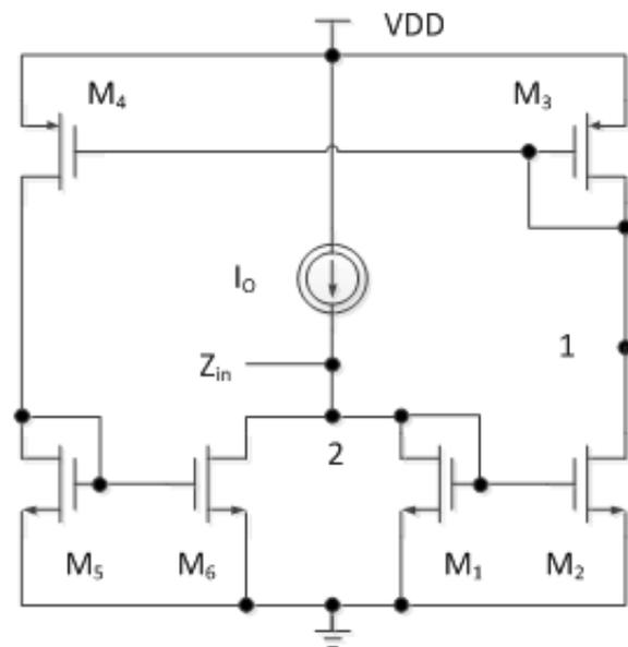
Fig. 1. Proposed current mode active inductor
