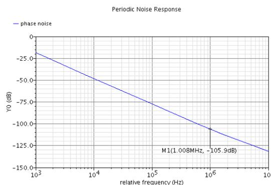
Fig. 7. The simulated phase noise at the oscillation frequency of 4.257GHz
