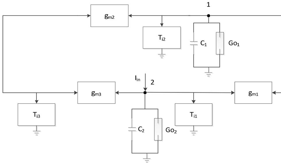
Fig. 2. equivalent network of the current mode active inductor
