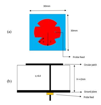
Fig. 1. Layout of the proposed antenna: (a) top view, (b) cross-sectional view
