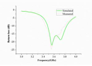
Fig. 7. Simulated and measured results for return loss at resonant frequency
