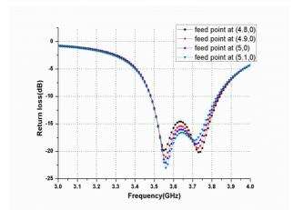
Fig. 3. Simulated return loss for the proposed antenna for different feed point locations
