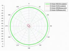
Fig. 11. 2D azimuth radiation patterns at 3.56GHz
