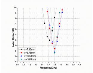
Fig. 2. Simulated axial ratio for the proposed antenna for different values of x
