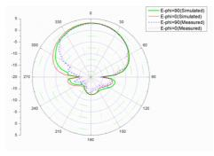
Fig. 10. 2D elevation radiation patterns at 3.56GHz
