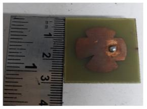
Fig. 6. Fabricated antenna designed at 3.56GHz
