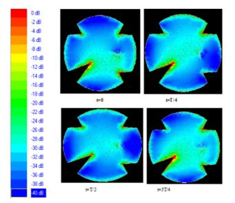
Fig. 4. Simulated current distributions of the proposed antenna at the resonant frequency of 3.56 GHz
