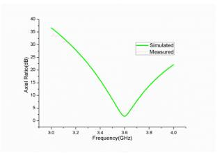
Fig. 8. Simulated and measured results for axial ratio at resonant frequency
