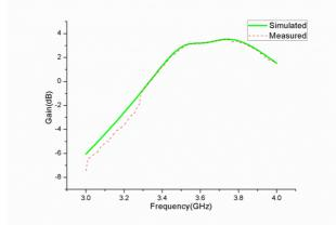
Fig. 9. Simulated and measured results for gain at resonant frequency
