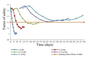
Fig. 13. Safety factor vs time at different rates of lowering of the reservoir, when the undrained shear strength of clay is 30kN/m<sup>2</sup>
