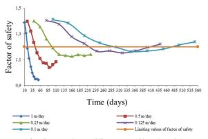
Fig. 10. Safety factor vs time at different rates of lowering of the reservoir, when the undrained shear strength of clay is 25kN/m<sup>2</sup>
