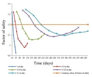
Fig. 7. Safety factor vs time at different rates of lowering of the reservoir, when the undrained shear strength of clay is 20kN/m<sup>2</sup>
