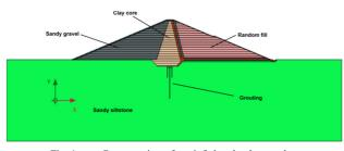
Fig. 1. Cross section of a rainfed embankment dam
