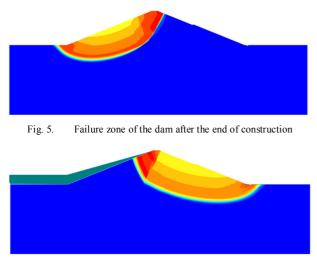
Fig. 6. Failure zone of the dam after the filling of the reservoir
