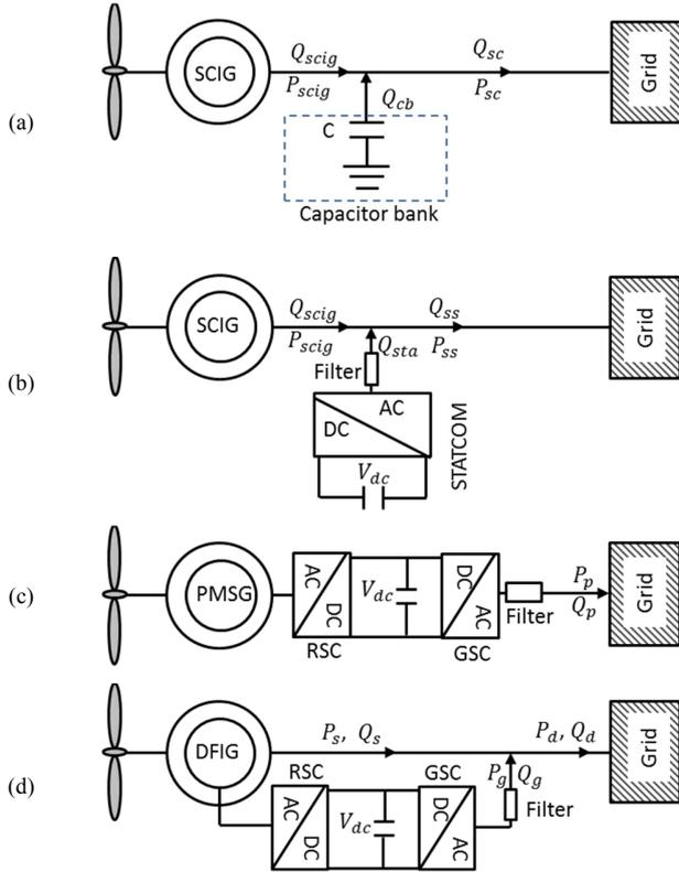
Fig. 1. Wind turbine configuration: (a) FSWT with capacitor bank, (b) FSWT with STATCOM, (c) FC-VSWT, (d) PC-VSWT
