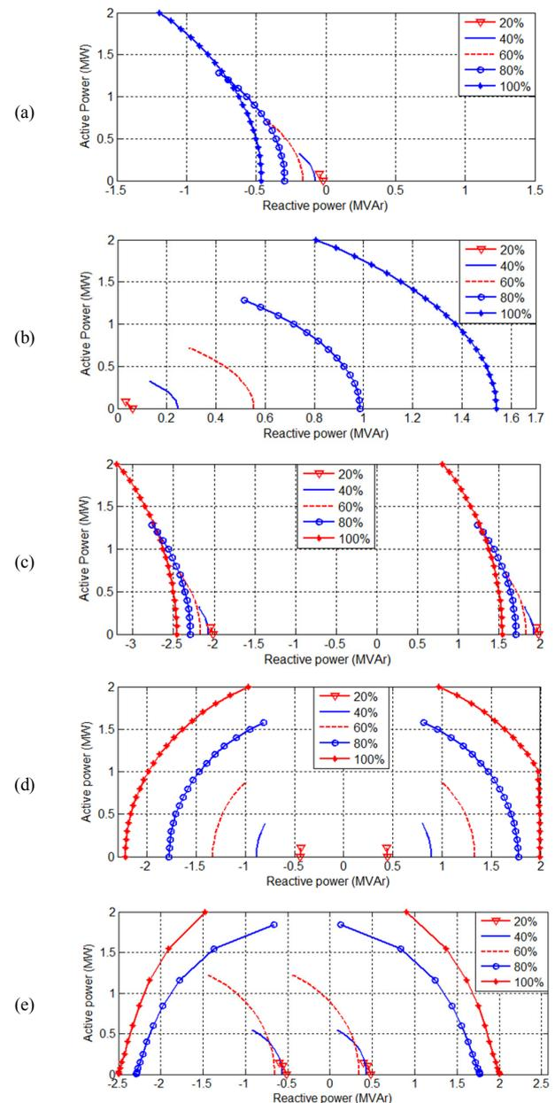
Fig. 4. Reactive power at voltage sag: (a) FSWT, (b) FSWT-capacitor bank, (c) FSWT-STATCOM, (d) FC-VSWT, (e) PC-VSWT
