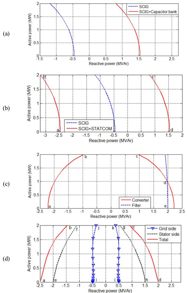
Fig. 3. Reactive power support capability in normal operation: (a) FSWT-capacitor bank, (b) FSWT-STATCOM, (c) FC-VSWT, (d) PC-VSWT
