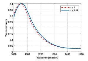
Fig. 10. Transmission characteristics of the sensor with three gratings with w=20 nm, d=250 nm, h=450 nm and n=1 and 1.01
