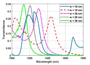
Fig. 5. Transmission characteristics of the sensor with h=400nm, d=250nm for different values of w
