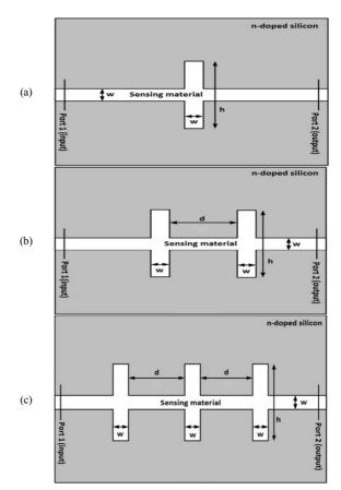
Fig. 3. The basic structure of the sensor with (a) single grating, (b) two gratings, (c) three gratings
