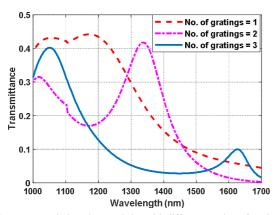
Fig. 4. Transmission characteristics with different number of gratings with w=20 nm, h=400 nm, and d=250 nm
