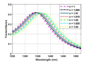
Fig. 8. Transmission characteristics of the sensor with w=20nm, d=250nm, h=450 nm for different values of n
