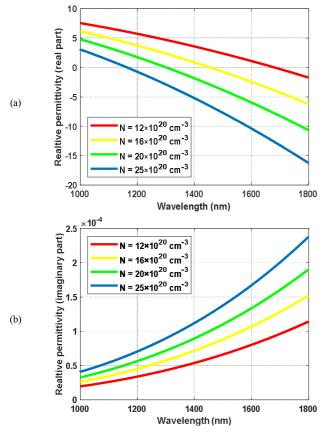
Fig. 2. Relative permittivity: (a) real part (b) imaginary part versus wavelength at different carrier concentrations
