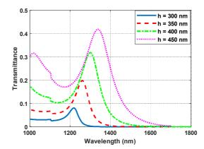
Fig. 7. Transmission characteristics of the sensor with w=20nm, d=250nm for different values of h
