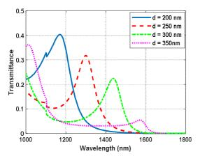
Fig. 6. Transmission characteristics of the sensor with w=20 nm, h=400 nm for different values of d
