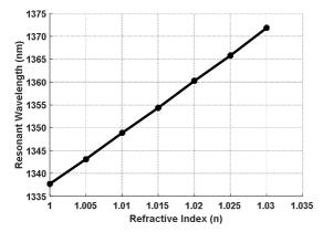
Fig. 9. Resonant wavelength shifts with the change of refractive index
