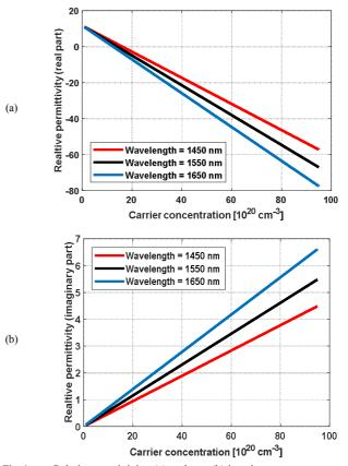
Fig. 1. Relative permittivity: (a) real part (b) imaginary part versus carrier concentration at different wavelengths
