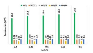
Fig. 5. Effect of tempering temperature after WQ on the corrosion rate of ASTM A-36 steel (using NaCl)
