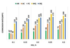
Fig. 1. Effect of the cooling rate after austenitizing treatment on the corrosion rate of ASTM A-36 steel (using HCI)
