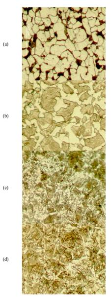
Fig. 7. Effect of different cooling rates on the microstructure of ASTM A-36 steel: (a) AR, (b) AC, (c) OQ and (d) WQ, X200
