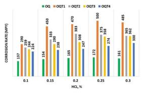
Fig. 3. Effect of tempering temperature after OQ on the corrosion rate of ASTM A-36 steel (using HCl)
