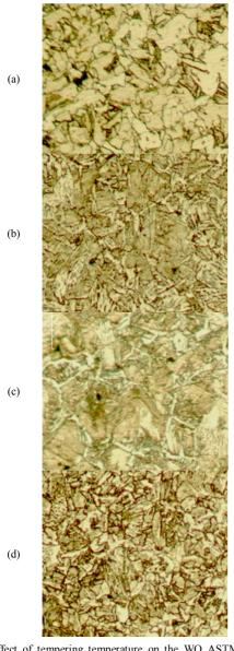
Fig. 8. Effect of tempering temperature on the WQ ASTM A-36 steel: (a) 250°C, (b) 350°C, (c) 450°C and (d) 550°C, X200
