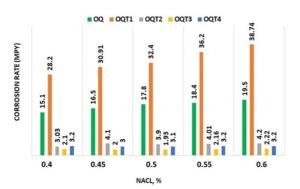
Fig. 6. Effect of temperature after OQ on the corrosion rate of ASTM A-36 steel (using NaCl)
