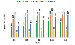
Fig. 2. Effect of tempering temperature after WQ on the corrosion rate of ASTM A-36 steel (using HCl)
