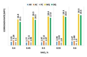
Fig. 4. Effect of heat treatment on the corrosion rate of ASTM A-36 steel (using NaCl)
