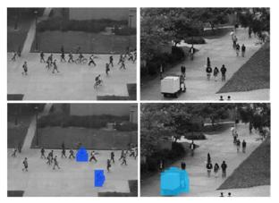
Fig. 3. The top row shows sample frames taken from four video sequences. The bottom row shows anomalous entities annotated and highlighted in different colors. Images from UCSD  ${\rm \bigcirc}$  SVCL
