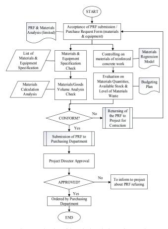
Fig. 1. Flowchart of the revised standard operating procedure
