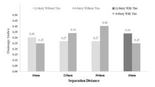
Fig. 6. RSN0020 weighted damage indices for adjacent building blocks with installation of tying devices
