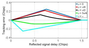
Fig. 1. Tracking error plot against signal's relative delay for a multipath signal with relative amplitude of 0.5 and varying carrier phase offsets ( $\varphi$ ) with respect to the LOS signal.
