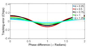
Fig. 4. Tracking error plot against signal's relative phase difference for a multipath signal with relative amplitude of 0.3 and varying multipath signal delay (*d*) with respect to the LOS signal.
