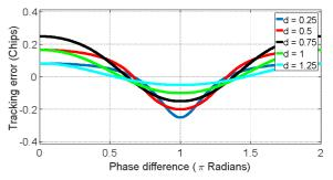
Fig. 5. Tracking error plot against signal's relative phase difference for a multipath signal with relative amplitude of 0.5 and varying multipath signal delay (d) with respect to the LOS signal.
