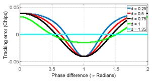
Fig. 12. Tracking error plot against signal's relative phase difference for a multipath signal with relative amplitude of 0.8 and varying multipath signal delay (d) with respect to the LOS signal, using narrow correlators in receiver.
