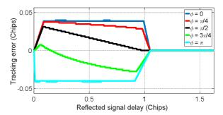
Fig. 9. Tracking error plot against signal's relative delay for a multipath signal with relative amplitude of 0.8 and varying carrier phase offsets ( $\varphi$ ) with respect to the LOS signal, using narrow correlators in receiver.
