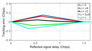
Fig. 2. Tracking error plot against signal's relative delay for a multipath signal with relative amplitude of 0.3 and varying carrier phase offsets ( $\varphi$ ) with respect to the LOS signal.
