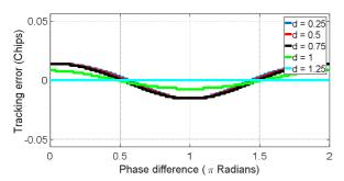
Fig. 10. Tracking error plot against signal's relative phase difference for a multipath signal with relative amplitude of 0.3 and varying multipath signal delay (d) with respect to the LOS signal, using narrow correlators in receiver.
