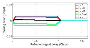
Fig. 8. Tracking error plot against signal's relative delay for a multipath signal with relative amplitude of 0.3 and varying carrier phase offsets ( $\varphi$ ) with respect to the LOS signal, using narrow correlators in receiver.
