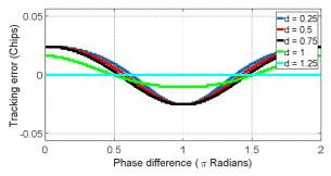
Fig. 11. Tracking error plot against signal's relative phase difference for a multipath signal with relative amplitude of 0.5 and varying multipath signal delay (d) with respect to the LOS signal, using narrow correlators in receiver.
