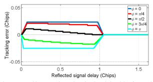
Fig. 7. Tracking error plot against signal's relative delay for a multipath signal with relative amplitude of 0.5 and varying carrier phase offsets ( $\varphi$ ) with respect to the LOS signal, using narrow correlators in receiver.
