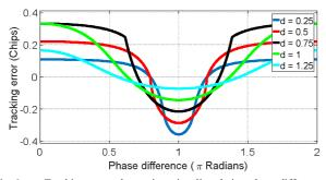
Fig. 6. Tracking error plot against signal's relative phase difference for a multipath signal with relative amplitude of 0.8 and varying multipath signal delay (d) with respect to the LOS signal.
