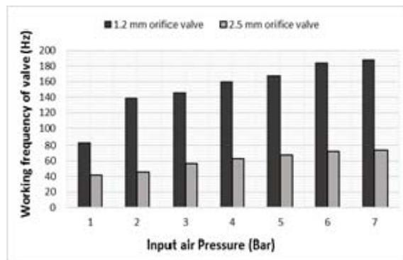
Fig. 4. Input air pressure Vs. Valve’s working frequency
