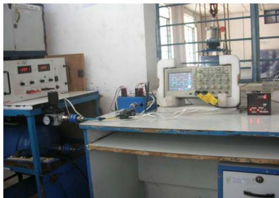
Fig. 2. Response time measuring unit
