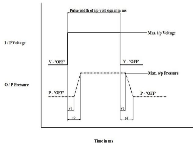
Fig. 1. Response Parameters Diagram
