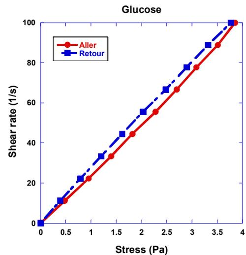
Fig. 2. Flow curves of the experimental results determine that the testing material is Newtonian.
