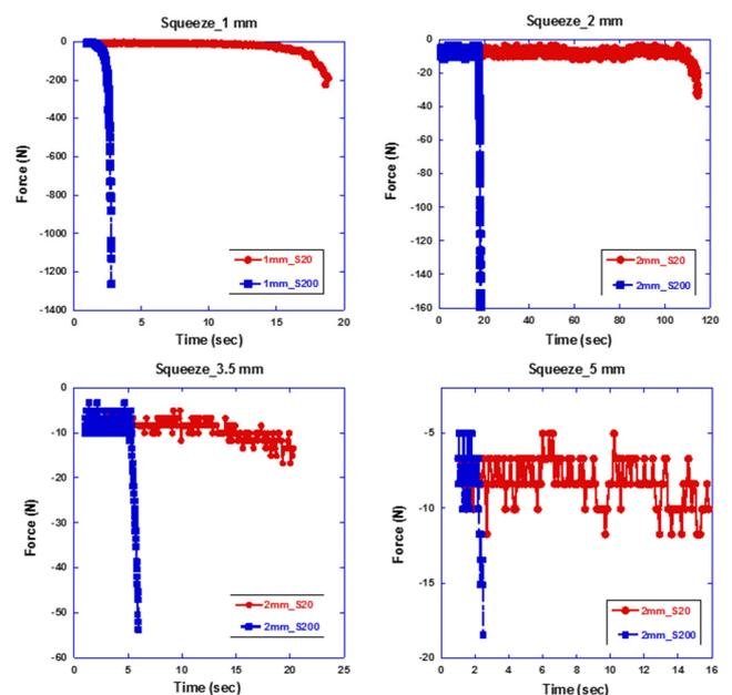
Fig. 3. The squeeze force obtained in the squeeze experiments.
