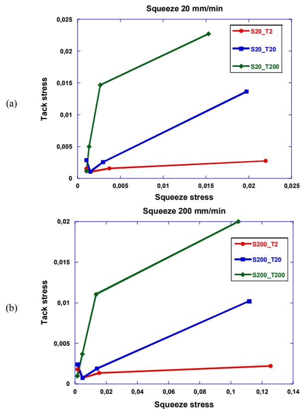
Fig. 6. Tack stress versus squeeze stress at different squeeze speeds.
