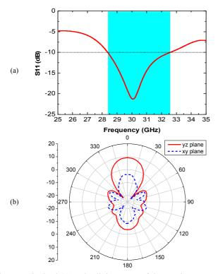
Fig. 7. Simulated S11 and radiation pattern of the two-element antenna array.
