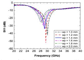
Fig. 5. Reflection coefficient with different antenna width wp.
