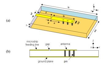
Fig. 1. Configuration of the single antenna: (a) perspective view, (b) side view.
