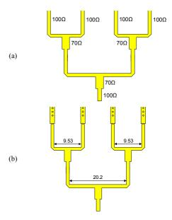
Fig. 3. The configuration of the four-element array: (a) 1:4 T-Junction power divider, (b) detail parameters.
