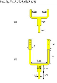
Fig. 2. Two-element antenna array: (a) 1:2 T-Junction power divider, (b) detailed parameters.
