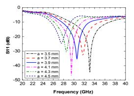
Fig. 4. Reflection coefficient with different DPS length a.
