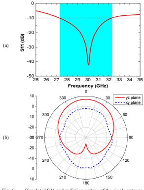
Fig. 6. Simulated S11 and radiation pattern of the single antenna.
