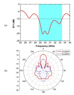
Fig. 8. Simulated S11 and radiation pattern of the four-element antenna array.
