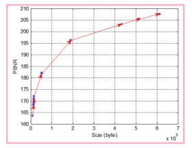
Fig. 7. PSNR as a function of image size.
