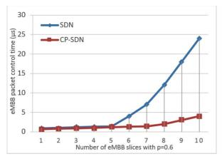
Fig. 8. eMBB delay performance for different values of n using the SDN and the CP-SDN at p=0.6.
