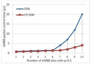
Fig. 7. eMBB delay performance for different values of n using the SDN and the CP-SDN at pA=0.5.
