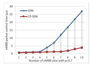
Fig. 9. eMBB delay performance for various values of n using the SDN and the CP-SDN at pA=0.7.
