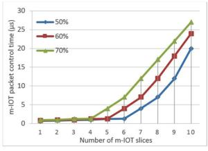
Fig. 6. m-IOT delay performance for different numbers of slices.
