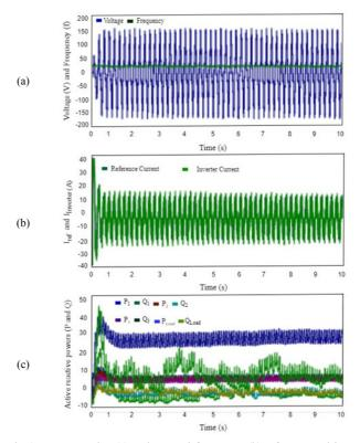
Fig. 9. IM results: (a) Voltage and frequency, (b) reference and inverter currents, (c) active and reactive powers.
