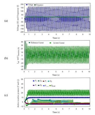
Fig. 7. GCM results: (a) Voltage and frequency, (b) reference and inverter currents, (c) active and reactive powers.
