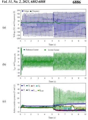
Fig. 10. Transition from IM to GCM: (a) Voltage and frequency, (b) reference and inverter currents, (c) active and reactive powers..
