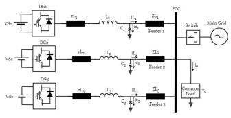
Fig. 1. A microgrid with three DG inverters connected in parallel.
