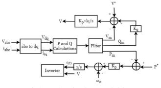
Fig. 4. Active and reactive power calculations.
