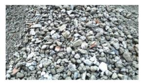
Fig. 2. Recycled coarse aggregates.
