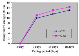
Fig. 4. Strength development of the recycled concrete.
