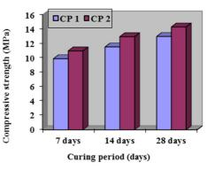
Fig. 5. Comparison of the strength of the two experimental recycled concrete mixes.
