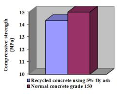
Comparison of the strength of recycled concrete using fly ash with Fig. 6. the conventional concrete.
