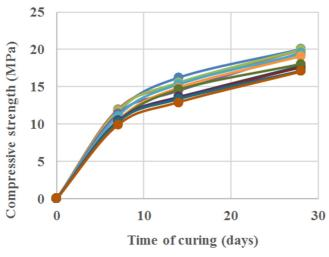
Fig. 4. The development of the compressive strength of concrete.
