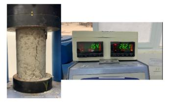
Fig. 2. An in-process experiment (CP20-28 days) and the recorded destructive force.
