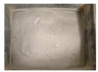
Fig. 1. Recycled fine-grained mixture obtained from crushed old concrete.
