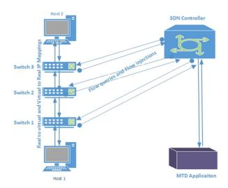
Fig. 2. Traffic flow sequence during IP mapping from real to virtual and vice versa.
