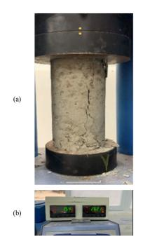
Fig. 1. (a) An in-process experiment (CP20) and (b) the recorded destructive force.
