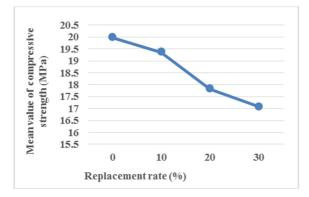
Fig. 3. Compressive strength of concrete at various replacement rates of natural fine aggregates with recycled fine aggregates.
