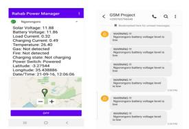
Fig. 7. Short message alert received from the system installed at Ngorongoro.
