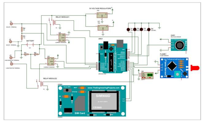
Fig. 1. Circuit diagram of the developed system.
