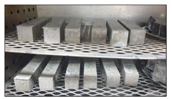
Fig. 5. Geopolymer prisms during curing.
