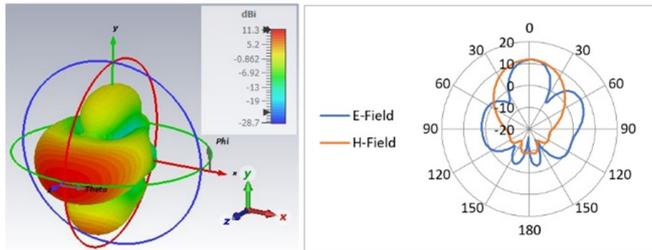
Fig. 4. The radiation pattern and E-H plane for the proposed antenna at 28GHz.
