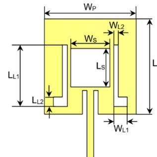
Fig. 1. Geometrical representation of the slotted patch element of the proposed microstrip antenna.
