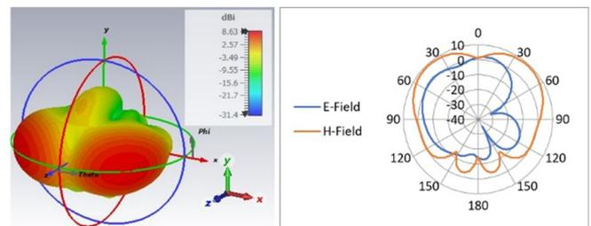
Fig. 3. The radiation pattern and E-H plane for the proposed antenna at 26GHz.
