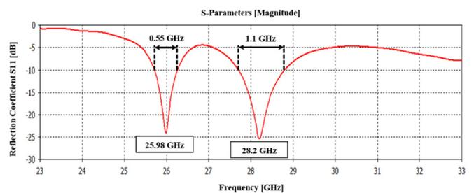
Fig. 2. S11 parameter as a function of frequency for the proposed antenna design.
