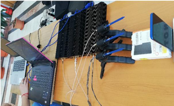
Fig. 1. Measurement ensemble with electric field probes, real-time spectrum analyzers, laptops, and the Motorola One 5G phone.
