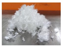
Fig. 1. Polypropylene fibers used in this work.
