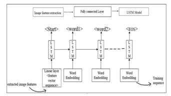
Fig. 7. Image vector to sequence the representation using the LSTM model.
