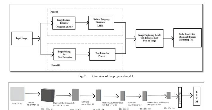
Fig. 3. Proposed D-CNN model followed by LSTM for image feature extraction.
