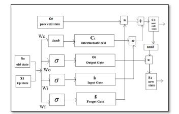
Fig. 8. Structure of LSTM.
