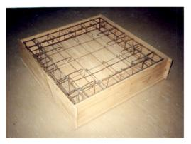
Fig. 1. The Reinforcement cage.
