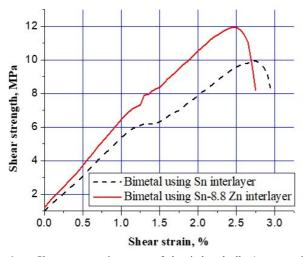
Fig. 6. Shear stress-strain curves of the tin-based alloy/gray cast iron specimens with Sn and Sn-8.8% Zn interlayer compositions.
