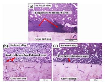
Fig. 4. Optical microstructure interfaces of tin-based alloy/gray cast iron specimens with different interlayer compositions: (a) flux only, (b) flux with Sn, (c) flux with Sn-8.8% Zn alloy.
