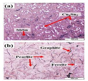
Fig. 3. Microstructures of (a) tin-based Babbitt alloy and (b) gray cast iron substrate, used for preparing the bimetallic casting.
