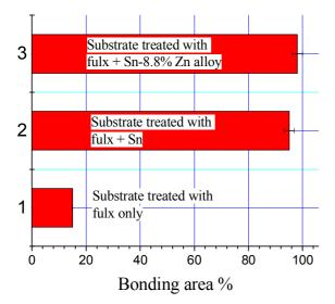
Fig. 5. Sn-based alloy/ gray cast iron bimetallic interfacial bonded areas as a function of interlayer pre-treatment compositions for the 3 sample groups.
