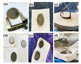
Fig. 1. Sn-based alloy/GG25 gray iron bimetallic casting: (a) gray iron substrate after cutting and grinding, (b)-(c) gray iron substrate during tinning with a hot plate, (d) gray iron substrates after tinning, (e) inserting the tinned gray iron substrate into the ceramic mold, (f) pouring the molten Sn-based alloy onto the ceramic mold.
