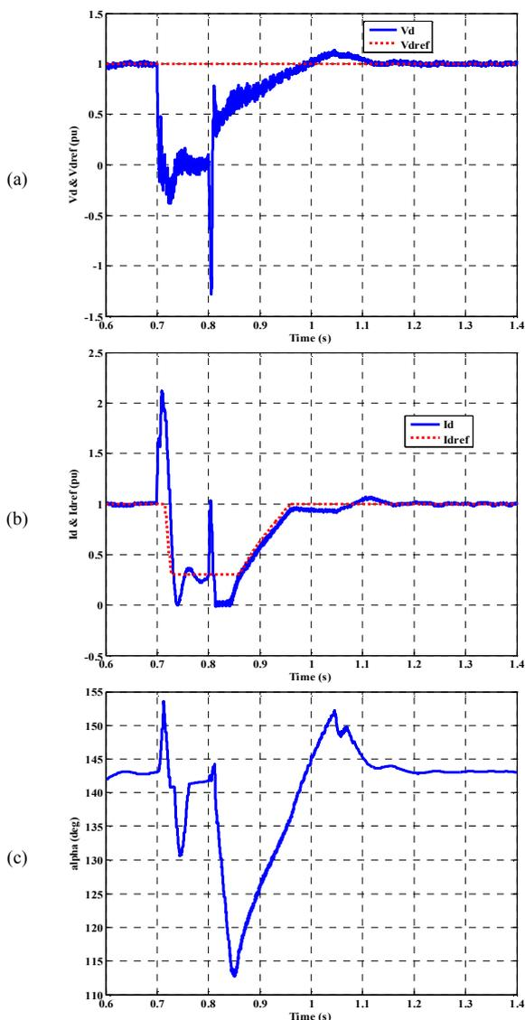
Fig. 4. Three-phase-to-ground AC fault on the inverter side.
