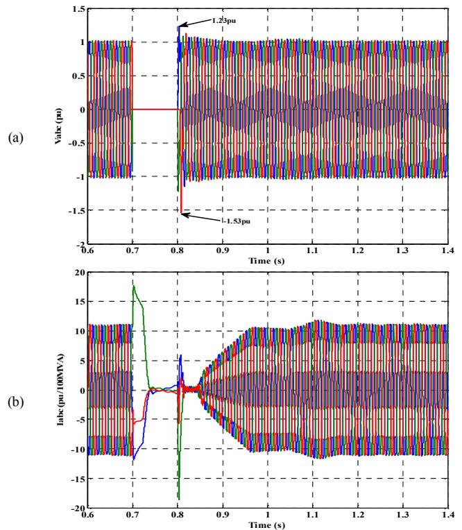
Fig. 5. Voltage and current responses under three phase to ground fault at the inverter.
