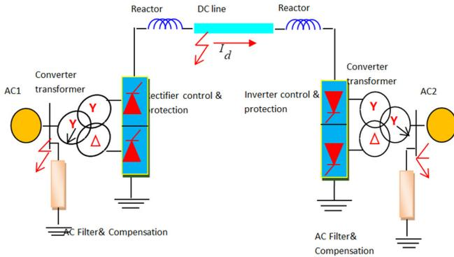
Fig. 2. Basic configuration of the HVDC transmission system.
