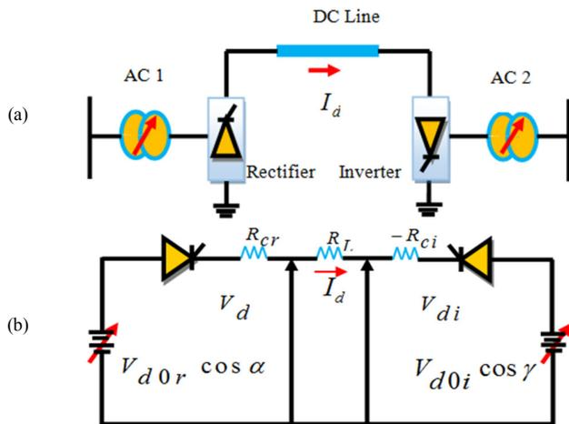
Fig. 1. HVDC transmission link: (a) schematic diagram, (b) equivalent circuit.
