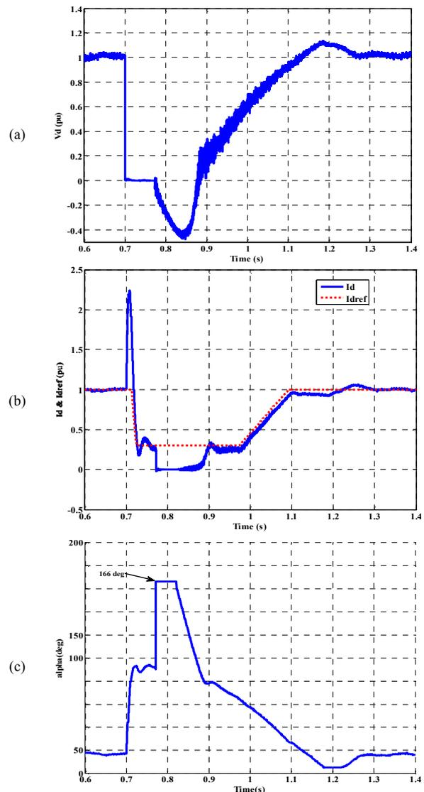
Fig. 3. DC fault on the rectifier side.
