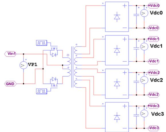
Fig. 7. Push-pull converter to create isolated DC sources.
