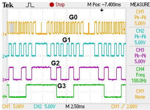
Fig. 13. Gate Pulses generated using ADC
