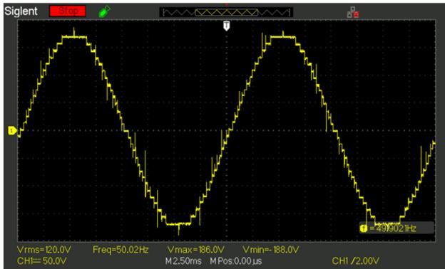
Fig. 14. Inverter output voltage at modulation index  $m=1.0$ .
