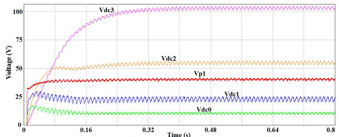
Fig. 8. Simulated output of the push-pull converter.
