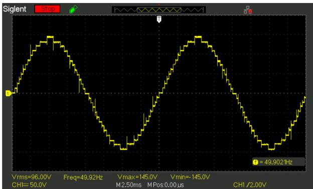
Fig. 15. Inverter output voltage at  $m=0.8$ .
