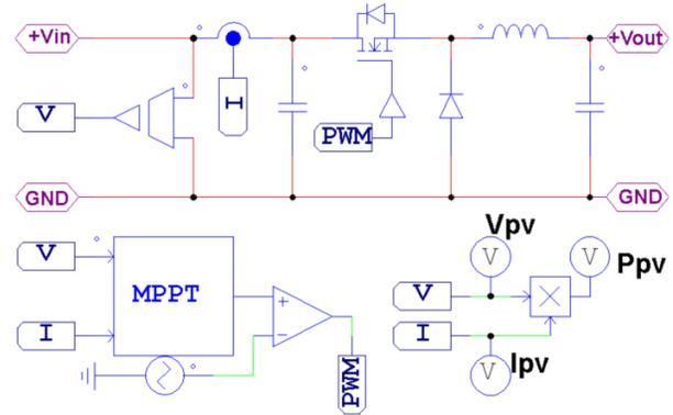
Fig. 6. Simulation diagram of the MPPT buck converter.
