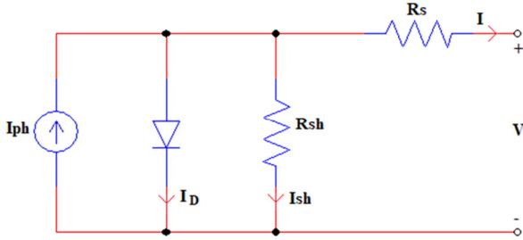
Fig. 2. Equivalent circuit for the PV cell.
