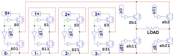
Fig. 9. Simulated power circuit of the 31-level inverter.
