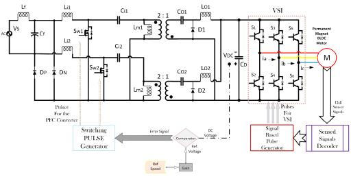
Fig. 1. Proposed isolated coupled Cuk converter-fed BLDC motor drive
