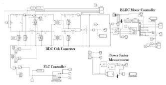
Fig. 8. Simulation diagram of the BDC converter with FLC.
