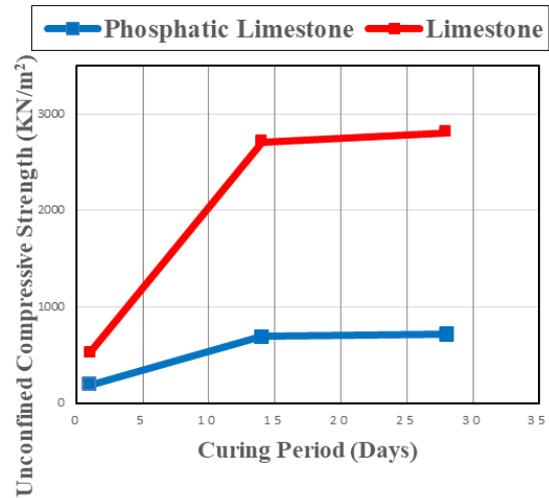
Fig. 9. UCS of samples cured for 1, 14, and 28 days.
