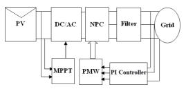
Fig. 1. The five-level inverter in grid-connected PV systems.
