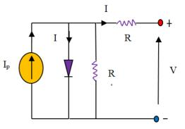
Fig. 3. Equivalent diagram of a photovoltaic cell.
