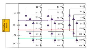
Fig. 2. The three-phase, five-level, diode-clamped inverter's schematic in Simulink.
